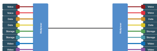
Multiplexing combines multiple channels on a single dark fiber
